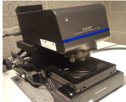
**Fig. 2.** LEXT™ OLS5000 SAF 3D Laser Confocal Scanning Microscope
